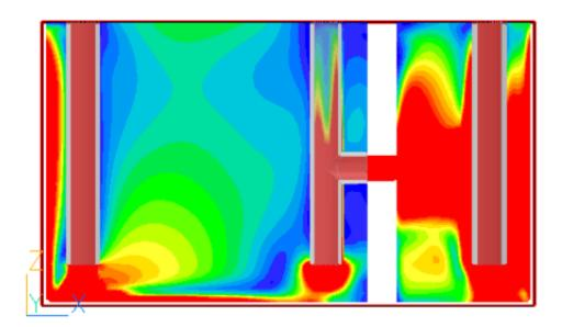
Short-circuiting from uncontrolled turbulence and velocity at 20 min RT
